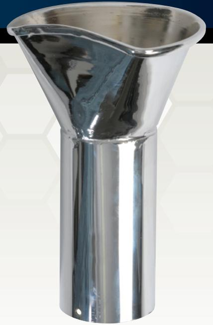
Copper and then Chrome Plated with approximately 0.4mm body and 1.0mm tail this product is for use in single and multi level structures as an access point to ensure proper drainage and to assist with locating blockages and has a flat back to securely fix to walls.
